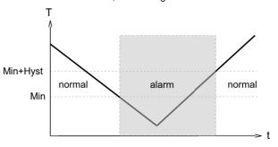
switchover to the alarm state. Return to the normal state occurs when the measured value once more falls below the limit value minus the set hysteresis.
