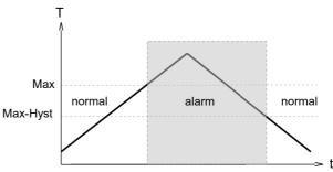
A changeover delay time  $(t_{DS})$  can be applied to switching to the alarm state. One switch-back delay time  $(t_{DR})$  of several can likewise be applied to switching back to the normal state.
