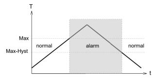
In the non-inverted (standard) model, while in the normal state the switching output is at the level of the supply voltage; in the alarm state it is at 0 V, so that a wire break would also display as an alarm state at the signal receiver. Optionally, an inverted switching output can also be provided, i.e. in the normal state the output is at 0 V, and in the alarm state it is at the level of the supply voltage.
