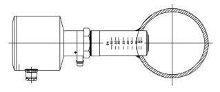
Weld on the nozzle at the marking according to its nominal width, free of distortion.
