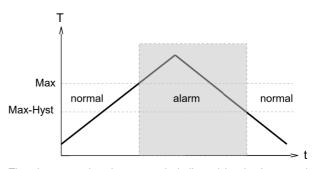
The change to the alarm state is indicated by the integrated red LED and a clear text in the display.
