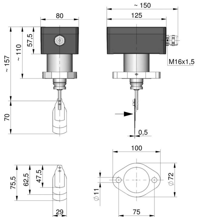
Paddle dimension and geometry are identical for DN 65; DN 80 and DN 100
