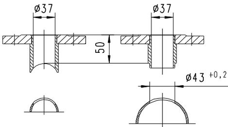
Pipe dimensions acc. to Din 2448 used for calibration at factory. Deviating installation conditions have an influence to set adjustment-/switching values.
